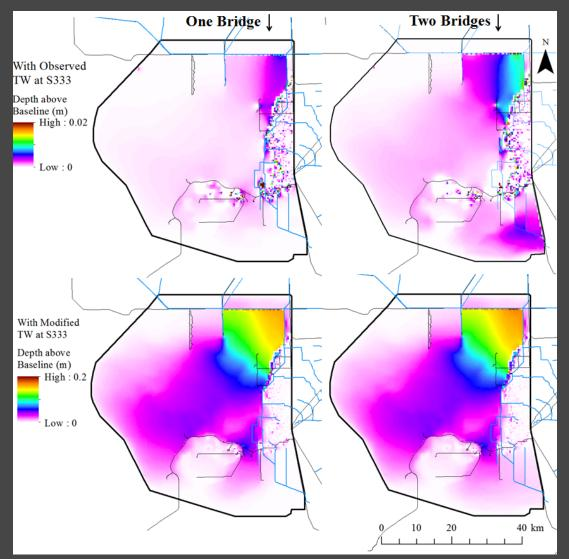
The modified tailwaters at S333 produced a gradient in the One Bridge and Two Bridge Scenarios which increased surface water levels (up to 21 cm) and hydroperiods more than bridge construction alone.
